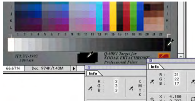
Comparing the 'infinite density' patch and the darkest gray scale RGB values
